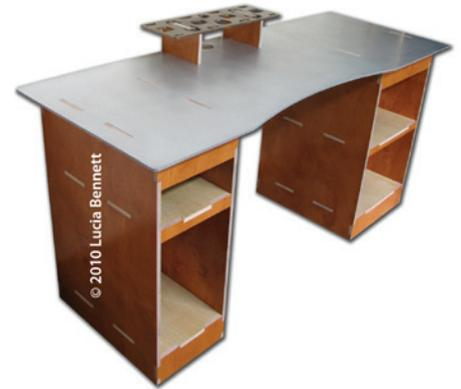
Above: A computer desk using box-joinery created on their waterjet. Made from Baltic Birch and aluminum.
