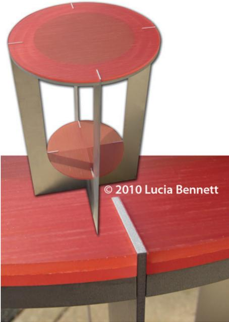
An interlocking table using tight kerf-widths and the OMAX Tilt-A-Jet®. Made from 3-Form® architectural recycled plastic and aluminum.
