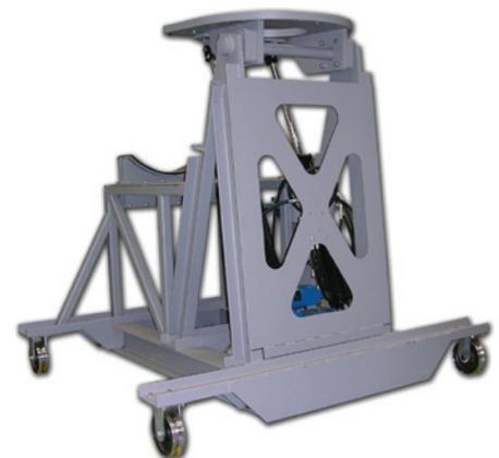
A hydraulic antenna tilt-stand for the U.S. Navy using waterjet cut 1/4", 1/2", 2 1/2" and 4" steel plate.
